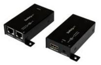
The ST121SHD30 HDMI® over CAT5e/CAT6 Video Extender kit lets you extend HDMI audio/video and an IR remote control signal by up to 100 feet (30 Meters) over dual Cat5e or Cat6 cable. For added versatility this HDMI extender kit is powered via the HDMI bus, and does not require any additional power adapter.
